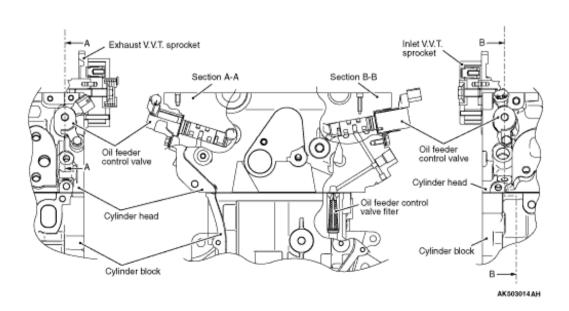
The MIVEC consists of the parts shown in the illustration.
