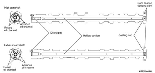
The camshaft is made hollow for weight reduction.
