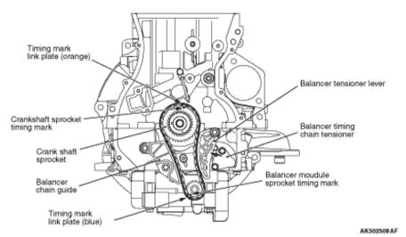
The balancer chain is a silent, endless type, consisting of 72 links. It is installed around the balancer module sprocket and the crankshaft sprocket. Two mark link plates (orange and blue) are installed on the balancer chain to locate the sprockets. When the balancer chain drives the balancer module sprocket, the balancer gear causes the right and left balancer shafts to rotate.
