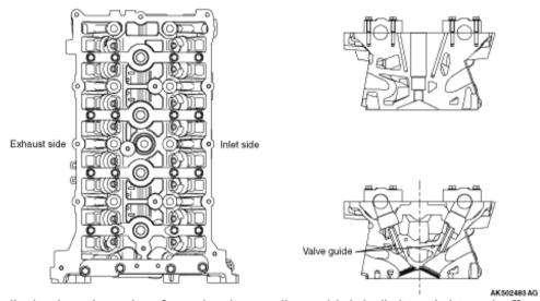
A cylinder head made of an aluminum alloy, which is lightweight and offers a high level of cooling efficiency, has been adopted. A pentroof combustion chamber with a center spark plug has been adopted. It has a small valve compound angle to realize a compact chamber.
