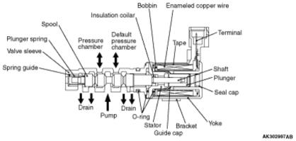
The oil feeder control valve consists of a solenoid valve, which switches the hydraulic pressure that acts on the vane rotor in the V.V.T. sprocket assembly. This valve is actuated by a signal from the engine ECU.
