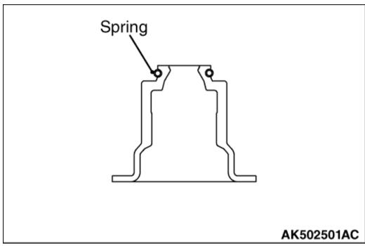
The valve stem seals are integrated with the valve spring seats.
