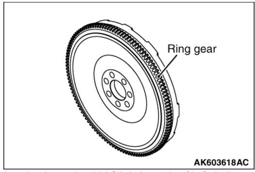
A cast iron ring gear is a shrink fit in the iron casting of the flywheel. The flywheel is mounted with 7 bolts.
