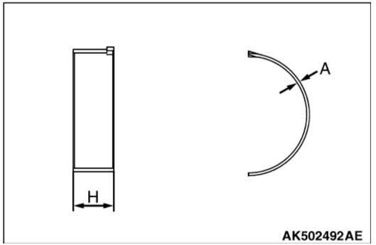
The upper and lower connecting rod bearings are the same. A connecting rod bearing is provided with a backing plate. Its bearing portion is made of an aluminum alloy and its backing plate is made of ordinary sheet steel.
