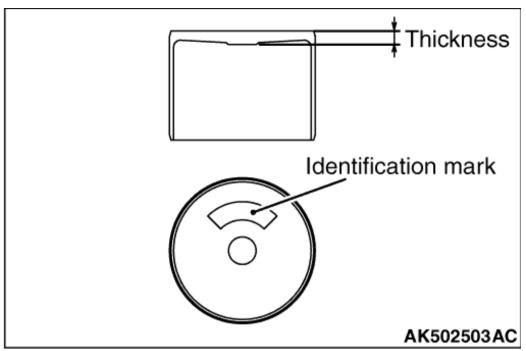
To adjust the valve lift, 47 sizes of valve tappets are available in 0.015 mm increments, from 3.000 to 3.690 mm.
