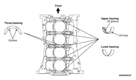
The upper crankshaft oil bearings have oil grooves and the lower crankshaft oil bearings do not have oil grooves. Each crankshaft bearing is provided with a backing plate. Its bearing portion is made of an aluminum alloy and its backing plate is made of ordinary sheet steel. A thrust bearing, which sustains the load in the thrust direction, is provided at each end of the No. 3 bearing.
