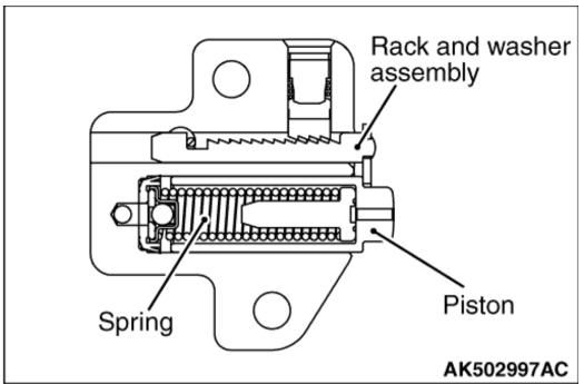
The tensioner maintains the tension of the timing chain. It contains a piston with a built-in spring.
