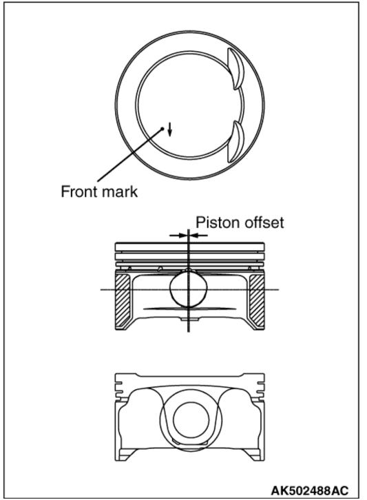
The pistons are made of a special aluminum alloy. Their weight has been reduced by lowering their overall height and increasing the depression at each
