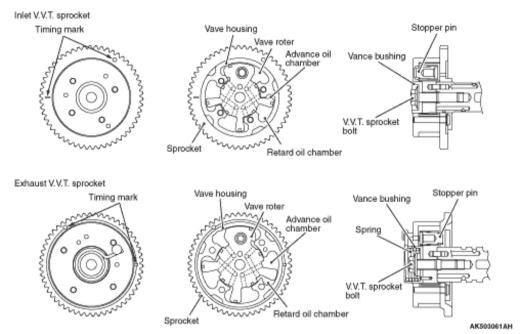
The hydraulic pressure that has been controlled by the oil feeder control valve acts to move the vane rotor in the V.V.T. sprocket, which is provided to optimally control the valve timing.
